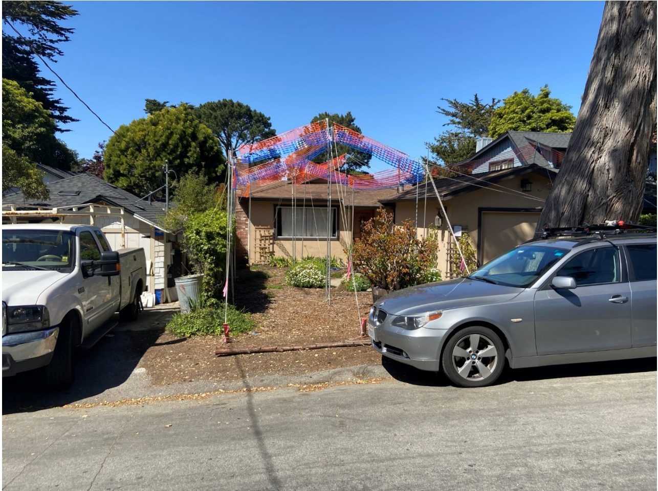
Figure 2. Garage story poles. Project proposal shown in orange with Applicant's proposed alternative shown in blue.
