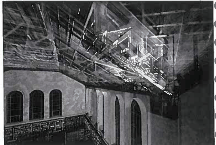
Laser technology provides accurate images of existing structure
