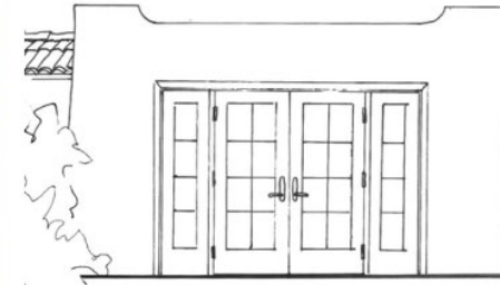
ADU conversion with French door infill retaining original garage door opening
