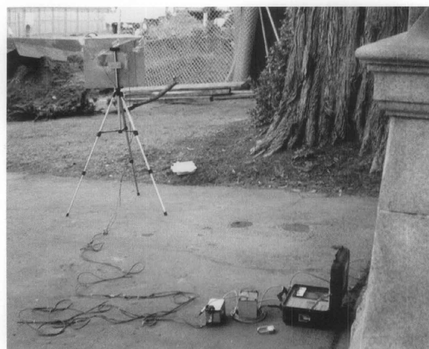
Figure 6. A seismograph records vibrations transmitted at the ground level of an historic building. The instrument is wired to a light and siren designed to warn the excavation crew that vibration levels are approaching preset limits. Additional sensors are often installed in the basement and on sensitive features such as stained glass windows. Photo: Wilson, Hirth & Associates, Inc.
