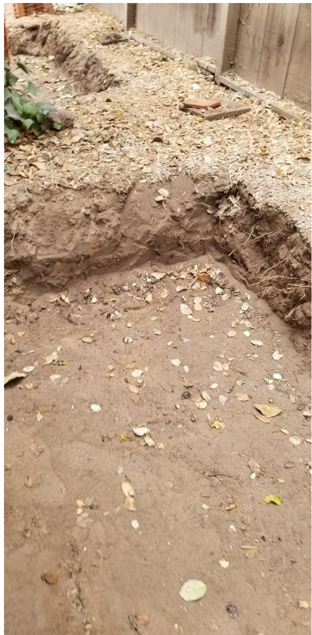
Figure 16: Excavated area near tree-12, roots up to 1-inches in diameter were found, along with many fibrous roots.
