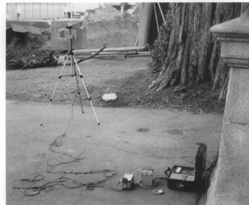
Figure 6. A seismograph records vibrations transmitted at the ground level of an historic building. The instrument is wired to a light and siren designed to warn the excavation crew that vibration levels are approaching preset limits. Additional sensors are often installed in the basement and on sensitive features such as stained glass windows. Photo: Wilson, Harg & Associates, Inc.
