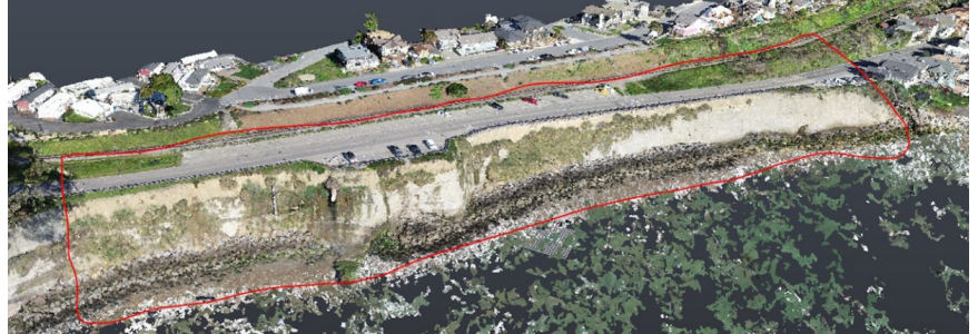
This is an example of a 3-dimensional model developed by CSW/ST2 for Cliff Drive in Capitola to support the planning of bluff stabilization. Using Autodesk® ReCap™, we can establish precise elevations along the entire bluff.
