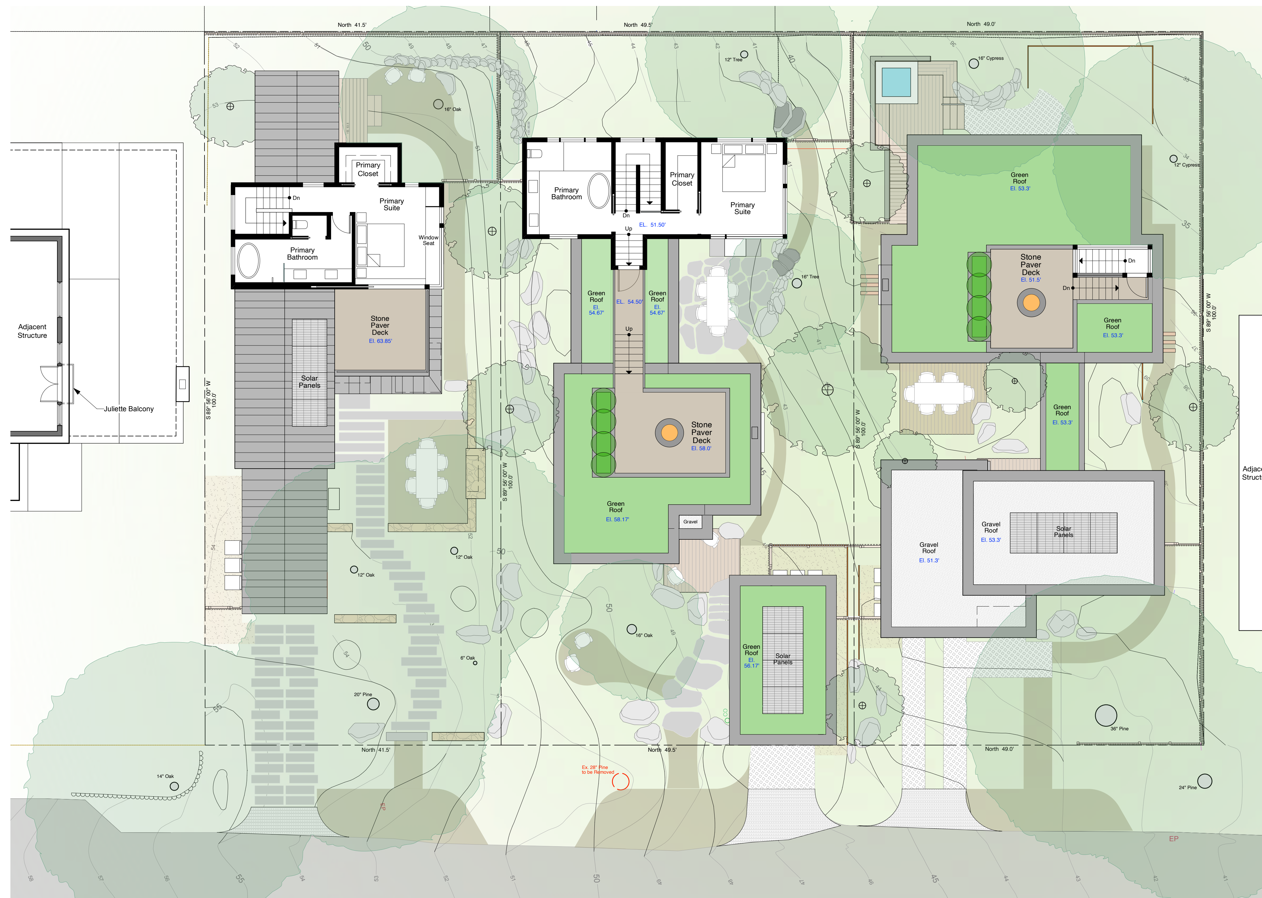
Overall Upper Floor Site Plan Scale: 1/8" = 1'-0"
