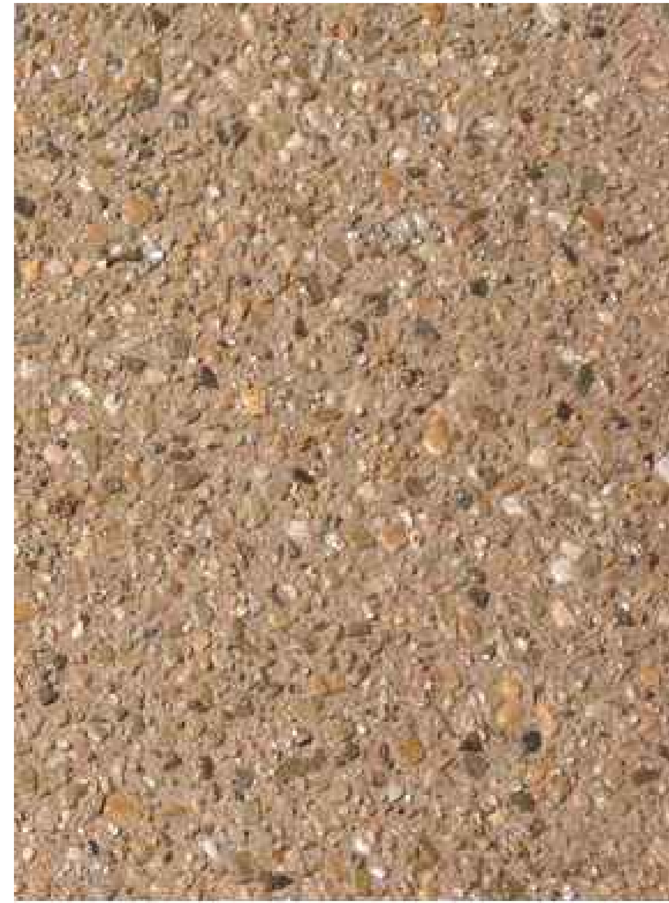
3 DRIVEWAY AND PATIOS AGGREGATE CONCRETE
