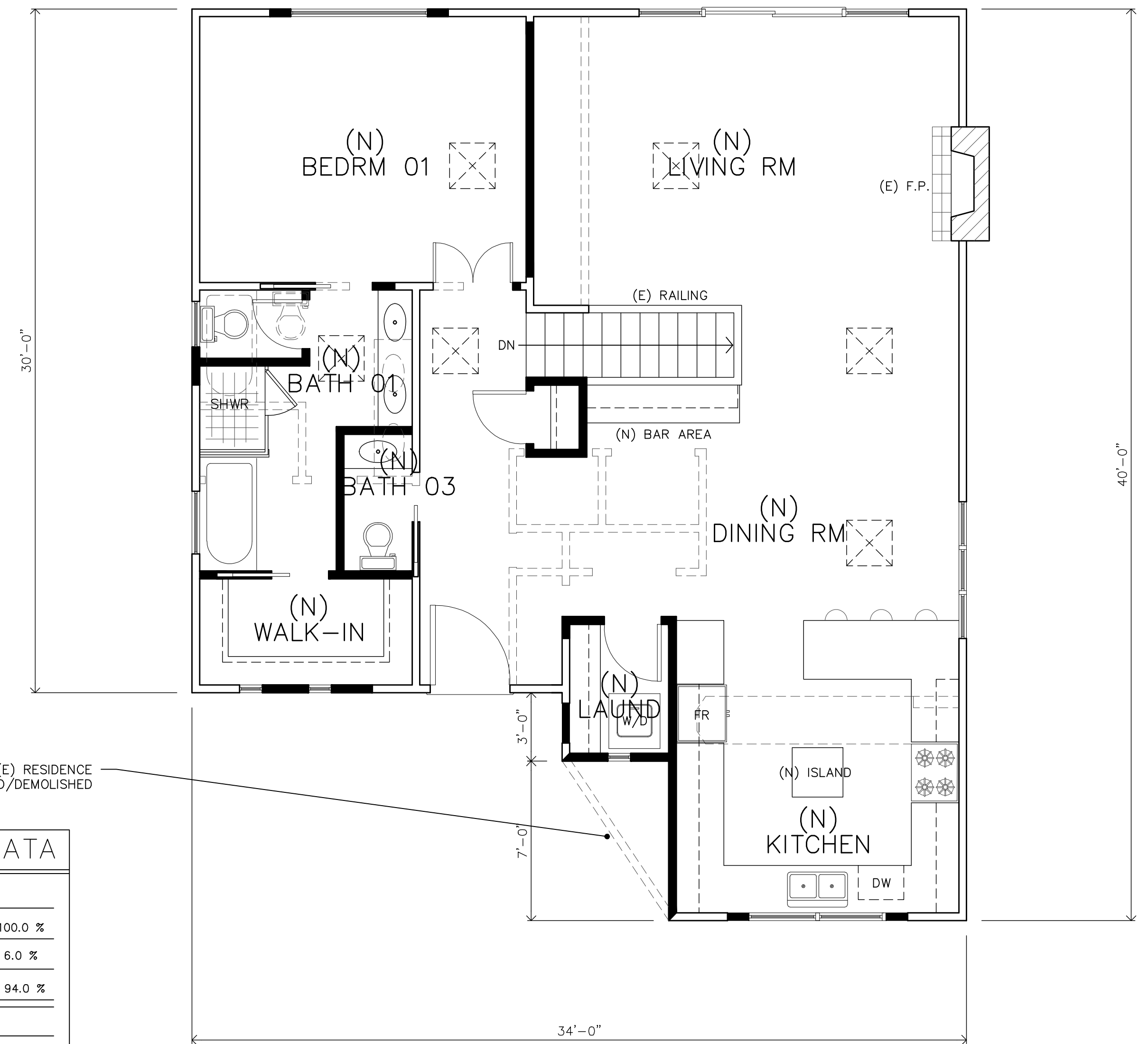
(E) MAIN LEVEL PLAN and DEMOLITION SCALE: 1/4"=1'-0"
