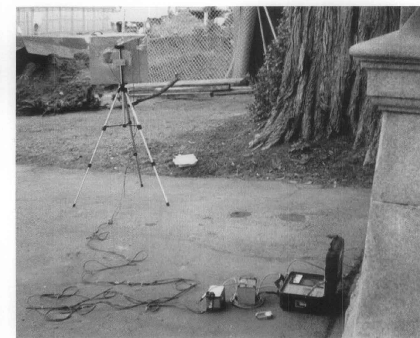
Figure 6. A seismograph records vibrations transmitted at the ground level of an historic building. The instrument is wired to a light and strobe designed to record the excavation crew that vibration levels are approaching preset limits.
